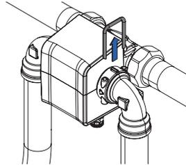
Pull the flexible hose with the connection elbow out of the connection flange of the CLEAR PRO SOFT TWIN.
