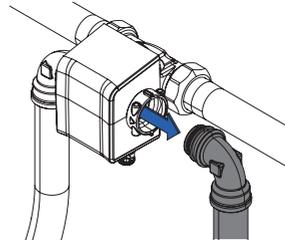
Insert the outlet fitting for raw water and secure the fitting with the clamps between the CLEAR PRO SOFT TWIN connection flange and the flexible hose with connection elbow.
