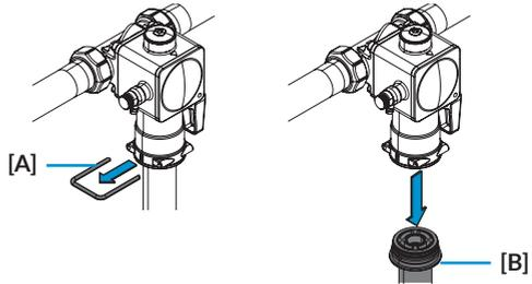
Fit the outlet fitting [C] for raw water to the connection flange from below and refit the clamp [A].
