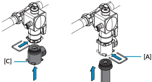
A pipe for direct water supply without treated water can now be connected to the side outlet.
