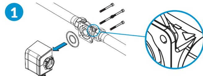
Mount the installation flange onto the already installed CLEAR installation flange.
