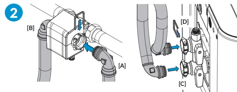
Connect the two armored hoses to the installation flange (armored hose raw water [A] at the inlet and armored hose soft water [B] at the outlet) and fasten the hoses with the clamps.
